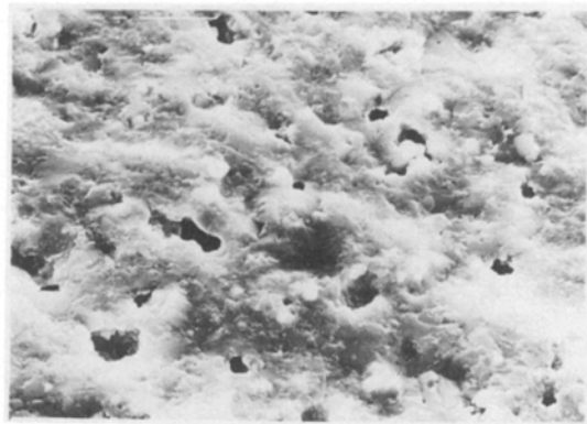
Fig. 4. Fracture surface of Nasicon which had been in contact with molten aluminium at 1073 K for 24 h. \times 0.9 K.
