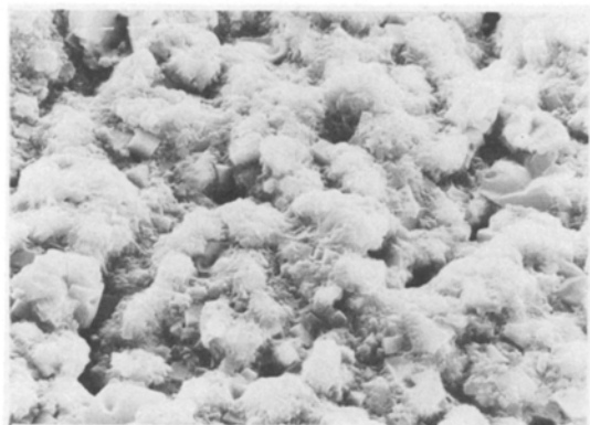
Fig. 3. Fracture surface of Nasicon sintered at 1433 K \times 0.9 K.
